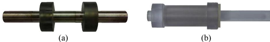
Figure 1: Projectiles for Split Hopkinson Pressure Bar test: (a) jig 1; (b) jig 2.
